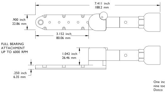
One inch 20 pitch thread with nine tooth spline drive adapts to Dotco American Pneumatic Buckeye Rockwell DeSoutter
