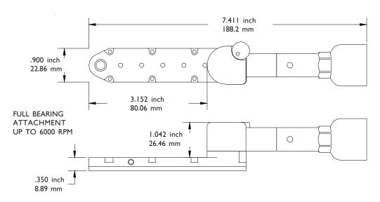
One inch 20 pitch thread with nine tooth spline drive adapts to Dotco American Pneumatic Buckeye Rockwell DeSoutter
